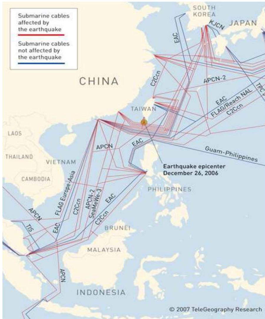
Even though many of these cable systems are SDH rings, **both parts of the ring pass through the Luzon Strait**, making ring-based restoration impossible when there is a large-scale submarine landslide in the strait
