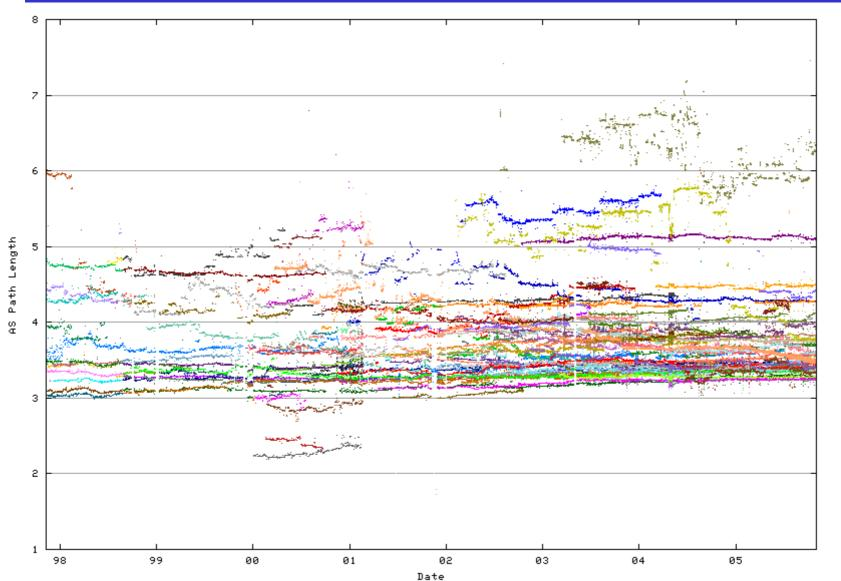
A constantly increasing number of ASNs can be related to average AS path length. The relatively constant AS path length for all AS paths implies that the density of AS interconnection is increasing at a rate proportional to the number of ASNs being added.
